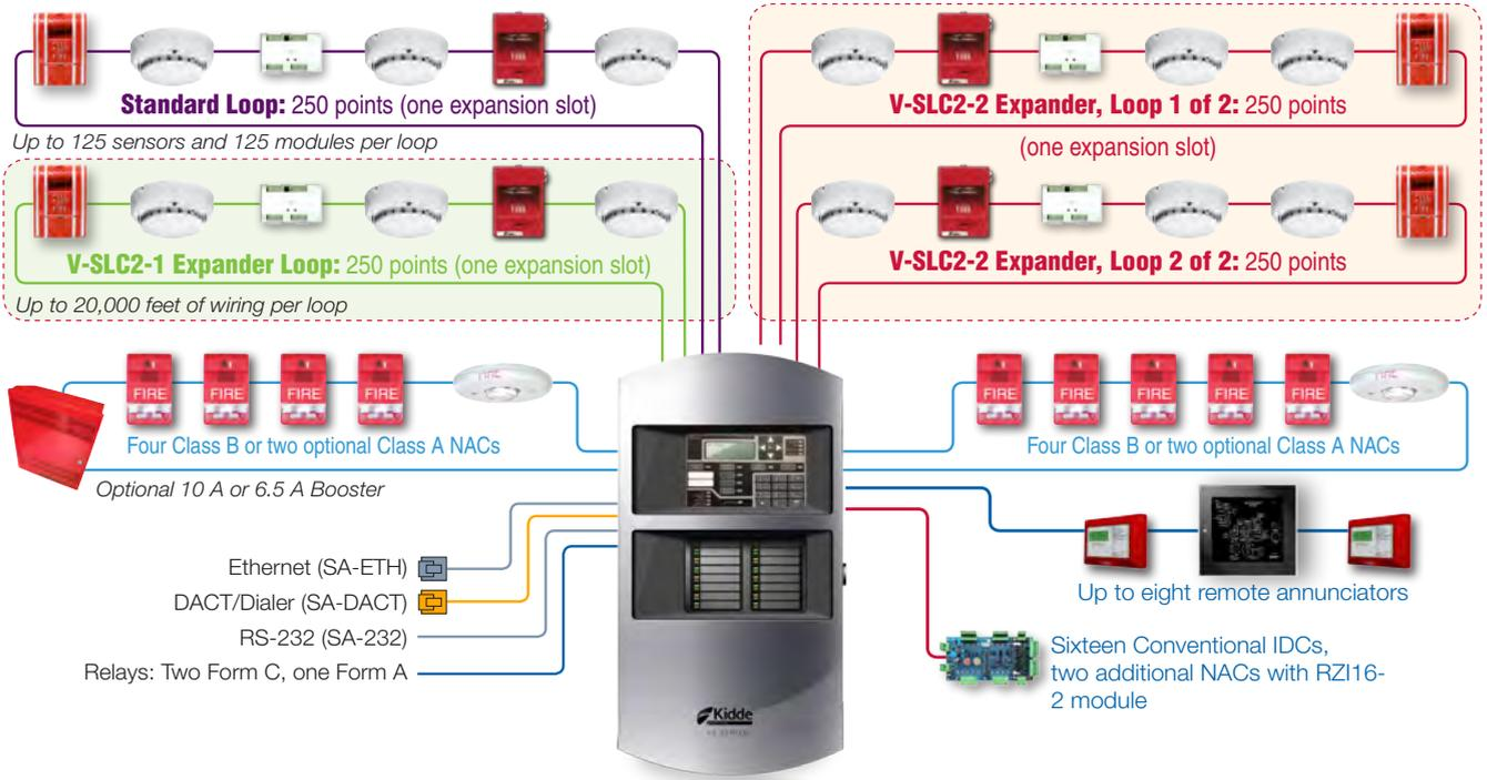
Each VS4 panel has room for up to two device loop controller modules in any combination of single or dual 250-device loops. VS4 comes with one loop that supports up to 125 detectors and 125 modules.
